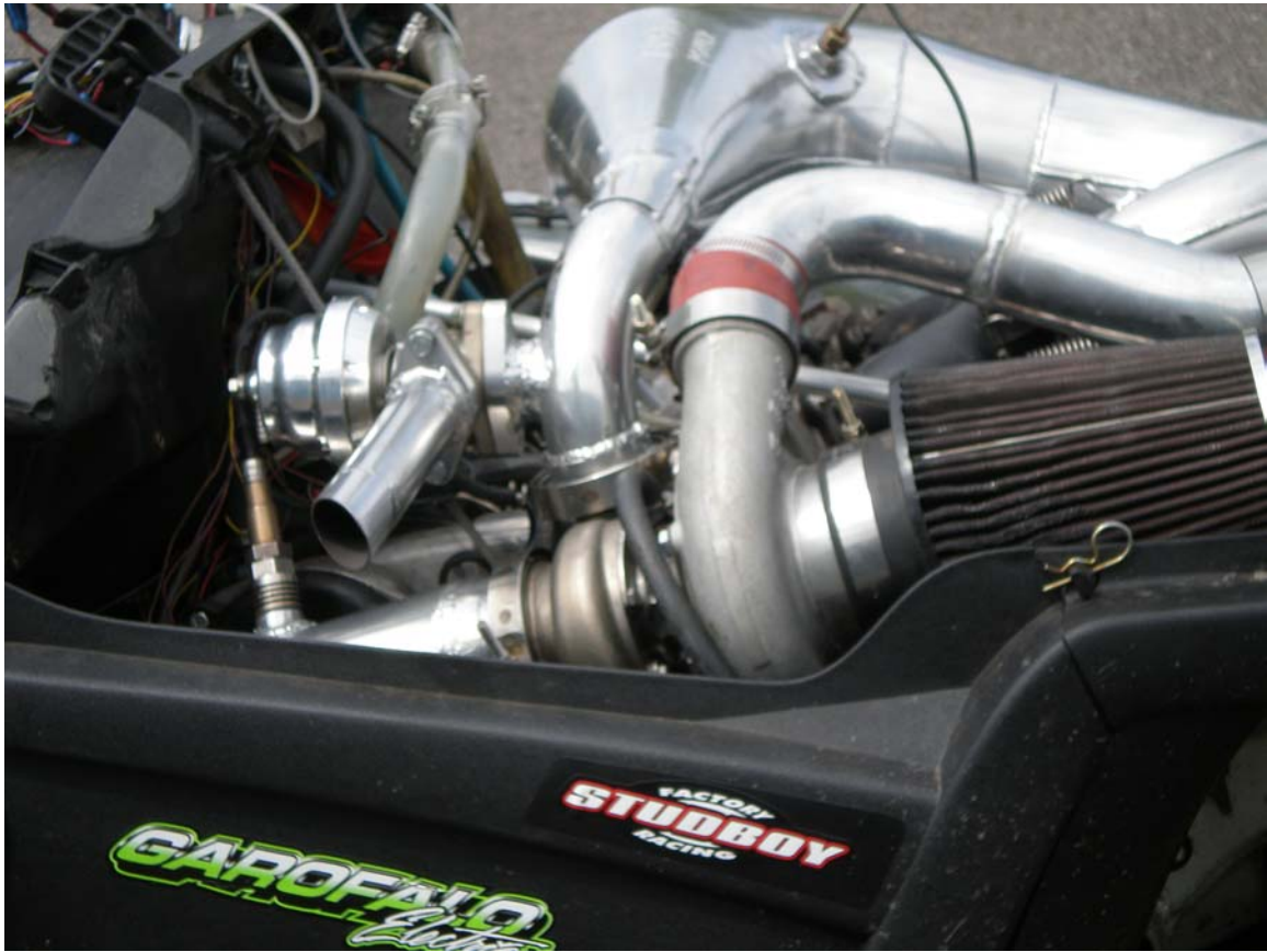
Here's the Big Dog Boondocker race turbo system, with D&D single pipe. Note the separate waste gate and clean stainless steel turbine housing.
