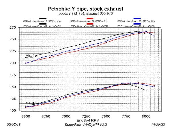
This was an early Petschke Ypipe left here years ago for testing by Billy Howard—a design that's since been taken over by D&D. I showed this one to Dale Roes and it's noticeably lower on HP compared to the first Petschke Etec 800 Ypipe tested by Chuck Hamarah and Steve Petschke back in 2011 (posted on this website). Dale sent me one of their production Y pipes, which is noticeably smoother internally. We'll test that one in Phase 3.
