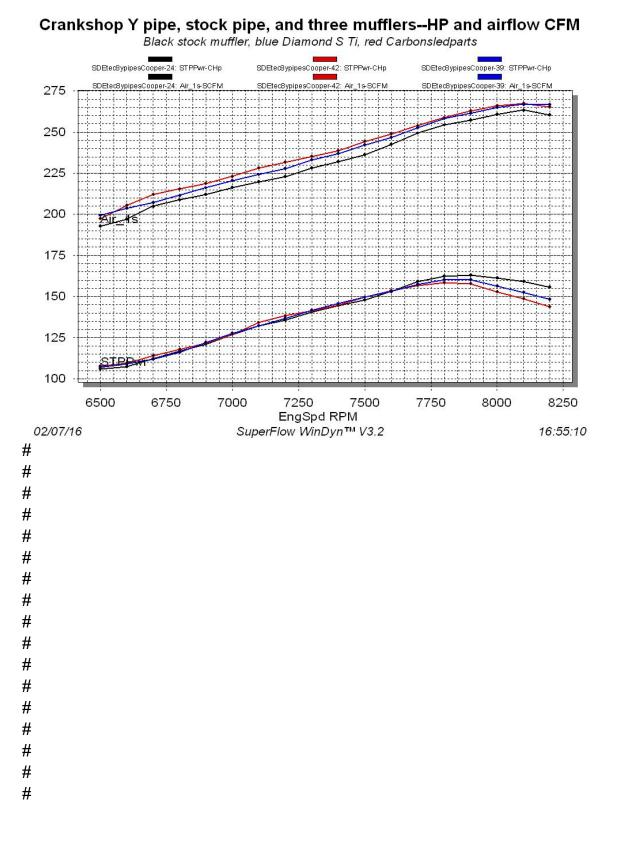
One final test was to reinstall the stock muffler and have Jim Cooper tweak the timing up to +3. Midrange HP was improved, but peak and overrev HP suffered a bit. So +2 is the best HP timing for this 2015 Etec 800.
