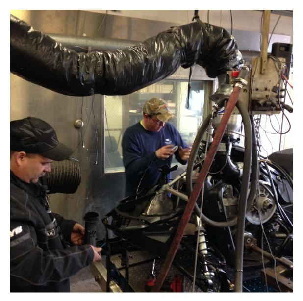
Here are Jim Cooper and Chad Giesler madly swinging wrenches. Note the insulated flexible duct feeding intake air from the cold room next door to the SuperFlow airflow meter attached to the stock air intake tube. When doing back-to-back, repeat dyno tests, even with 80mph outside air blowing at the sled, inadvertent EGR (exhaust gas recirculation) can sap HP and skew results. The cold room's replacement air comes from the roof of the building.
