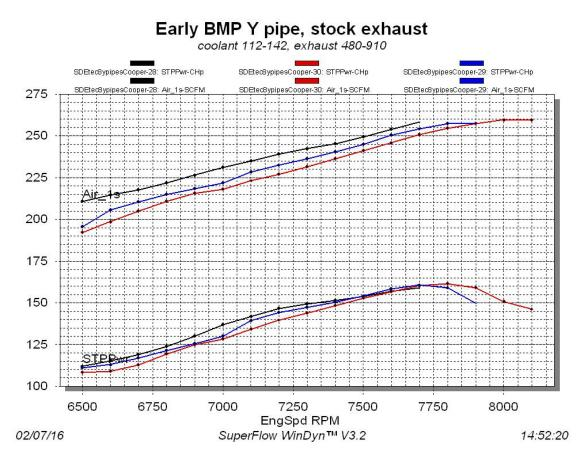
This BMP Y pipe has round, sanded exhaust port inlets. The newer BMP are said to have tapered tubes that are more oval shaped, and we'll try to obtain one of those for Phase 3 as well. As the final graphs show, this one was longest and had the best midrange HP improvement of all the Y pipes.
