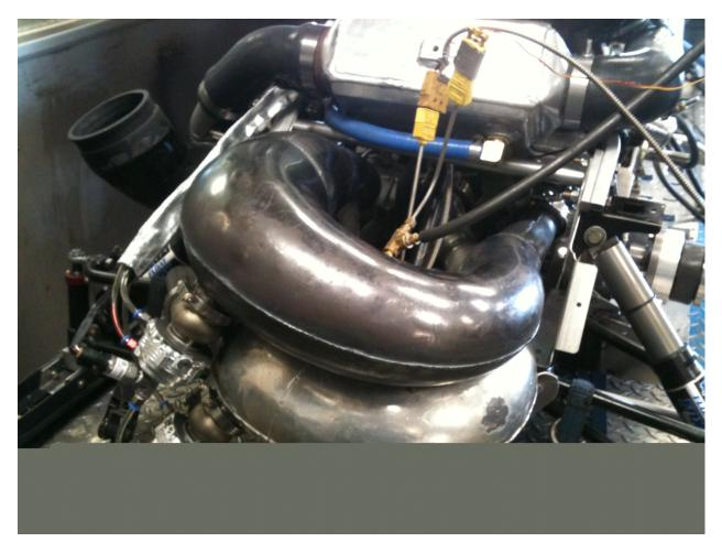
Here's the Mach Z turbo again—this time with twin pipes feeding the big Garrett ball bearing turbo. Separate wastegates are attached to each pipe. The odd brass T fitting on the top pipe's centersection allows dyno measurement of exhaust backpressure (for assessing turbine sizing) and temperature (to assure proper mixture from carb to carb, and determining what RPM peak HP will occur at).
