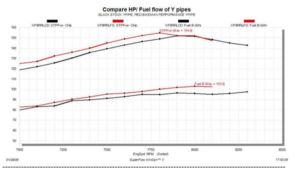
Next Jim Cooper used his computer to first advance, then retard timing in small increments. In this case, the stock factory zero setting delivered the maximum HP.
