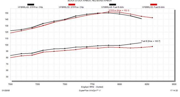
We installed, dyno tested then afterwards removed an MPRP can muffler because it appeared to increase airflow (note the higher fuelflow), and the reduced restriction/ backpressure was not optimal for 15 seconds at WOT and HP dropped by one. Due to the new for 08 internal stinger in the stock single pipe, noise output was not as bad as with previous non-internal stinger pipes.
