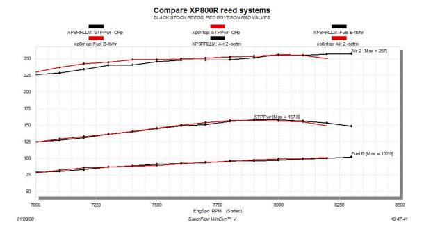
The sled owner was hoping for 160 HP after all of this, and since we were out of parts to try we reduced fuel flow from 97 to 94 lb/hr by dropping mains from 440 to 410. **Reduce main jet size from 440 to 410**
